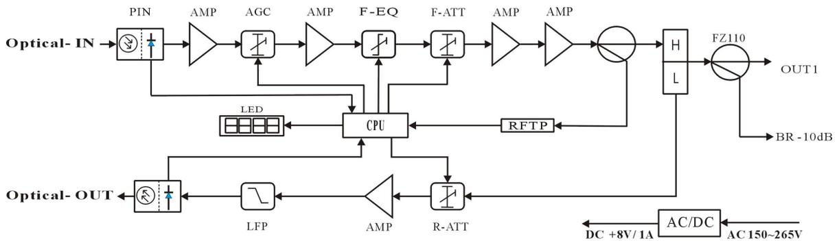
SR1002 without network management transponder, FP204 (two-way splitter) output block diagram
