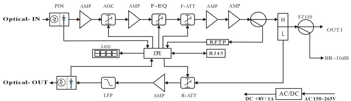
SR1002 with II class network management transponder, FP204 (two-way splitter) output block diagram
