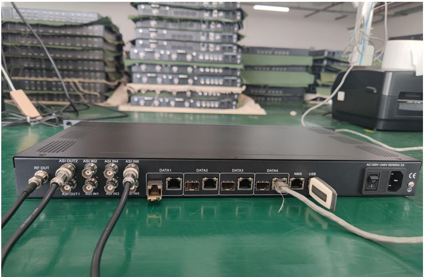
(Interface Connection Picture with ASI+IP+USB+SFP+RF)
